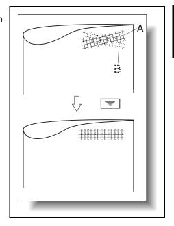
9 If horizontal lines A and B are angled as shown at the right, touch to specify the desired positive adjustment for θ (between +1 dot and +10 dots).
